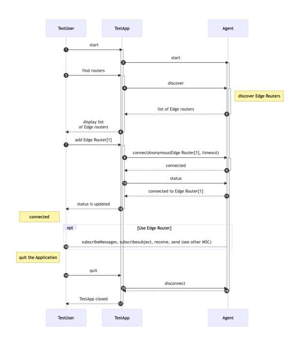
Figure 7 – UML MSC Diagram: MMS Agent connects anonymousely to an MMS Edge Router from User/App point of view.
