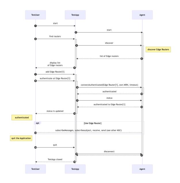
Figure 8 – UML MSC Diagram: MMS Agent connects and authenticates to an MMS Edge Router from User/App point of view.
