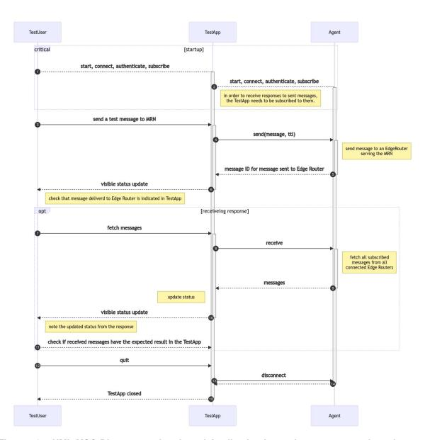
Figure 12 – UML MSC Diagram: authenticated Application is sends messages and receives response.
