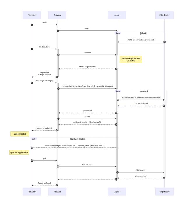
Figure 13 - UML MSC Diagram: MMS Agent connects and authenticates to MMS Edge Router from User/App point of view.
