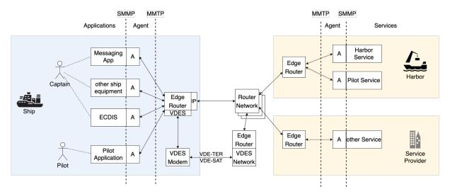
Figure 3 – Overview of MMS system architecture with VDES connection.
