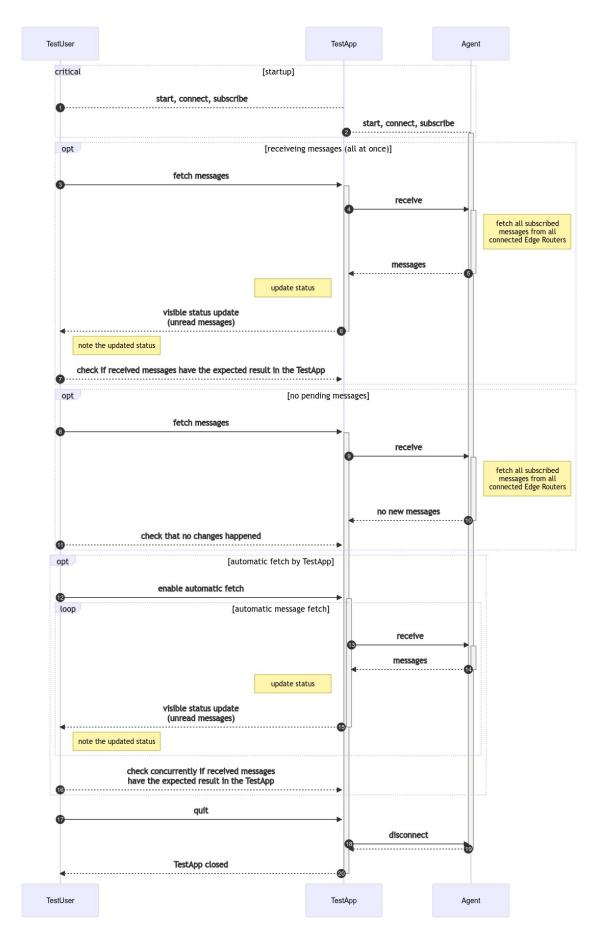
Figure 11 – UML MSC Diagram: MMS Agent receives messages.
