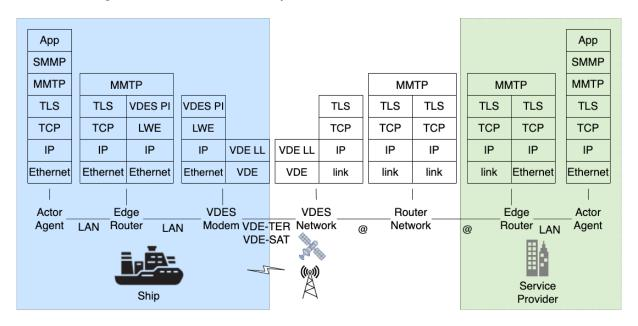
Figure 4 – Example of MMS protocol layering for messages over VDES.
