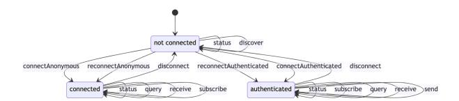
Figure 6 – UML diagram showing the functionality of the MMS Agent.
