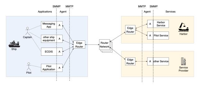
Figure 1 – Overview of MMS system architecture.
